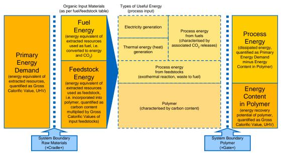
Energy flow diagram showing how primary energy demand (system input) is disproportioned into fuel and feedstock energy (within system), and process energy and energy content in polymer (system output)
