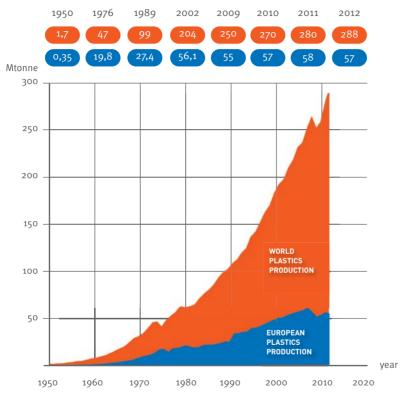
Figure 2: World plastics production 1950-2012 Includes thermoplastics, polyurethanes, thermosets, elastomers, adhesives,
